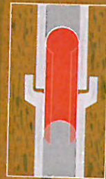
Collar repair with short liner
