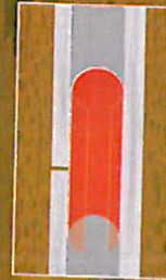
Crack repair with short liner
