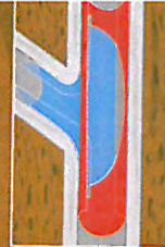
Joint with short liner and insert technology
